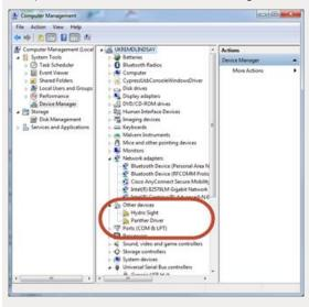
The Panther Driver relates to the operation of the Hydro Sight camera. This device can use a generic windows driver, so it may be removed from the warning list.
