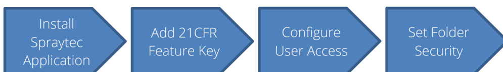
Figure 1. Typical installation process required for validated systems.
