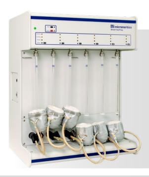
The Micromeritics Smart VacPrep™ 067 is an advanced six-port system that utilizes vacuum to prepare samples by heating and evacuation. Each of the ports may be operated independently. Samples may be added or removed from degas ports without disturbing the treatment of other samples undergoing preparation. Degassing automatically terminates when the samples have completed all programmed steps.
