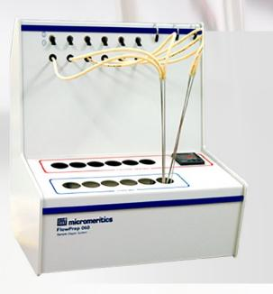
The Micromeritics FlowPrep O6O applies both heat and a stream of inert gas to the sample. The heat causes contaminants to desorb from the surface and the stream of inert gas sweeps them out of the sample tube. The unit lets you choose the temperature, gas, and flow rate best suited for your sample material and application. Needle valves allow you to introduce the flowing gas slowly to prevent fluidization of samples.
