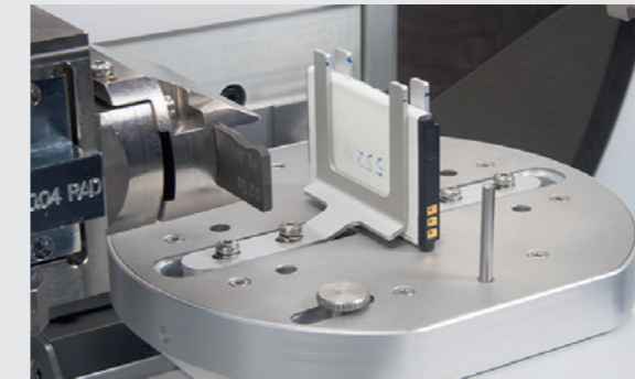
Pouch and prismatic cell mounting on the Empyrean XRD. A mechanism to apply pressure on the pouch cell is also supported.
